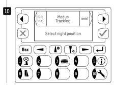
II If season mode is selected the last screen allows you to define a date frame in which the system moves into SIPO2 instead of SIPO1 to avoid problems with heavy snow
