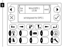
ID The next settings is used to program the position in which the unit stays during the night (tracking/SIP01/SIP02/season)
